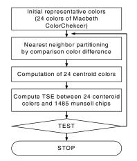
Figure 2. Application of Lloyd algorithm for building subpopulations of spectral reflectance.
