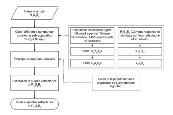
Figure 1. Flowchart of the proposed surface spectral estimation using set of principle components separately organized for each population of spectral reflectance.
